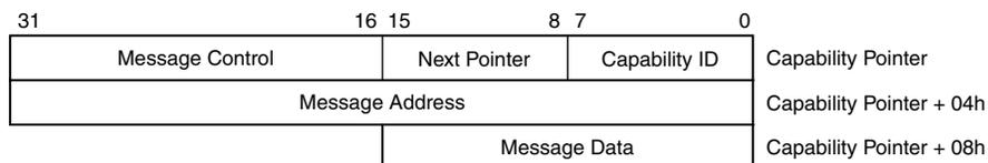
Capability Structure for 64-bit Message Address
