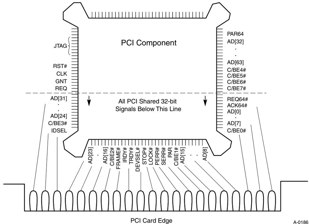
**Figure 4-9: Suggested Pinout for PQFP PCI Component**
