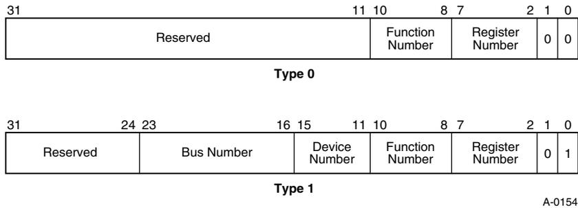
**Figure 3-1: Address Phase Formats of Configuration Transactions**
